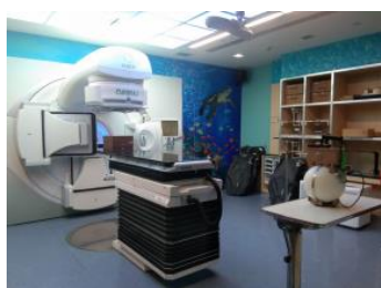
Figure 1. The equipment set-up for measuring neutron dose rate at location 2: the distal end of the couch
