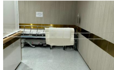
Figure 2. Placement of CR-39 dosimeters in air in treatment room.
