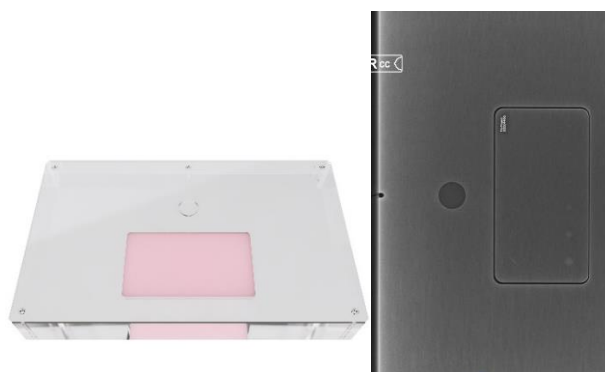
Figure 3. ACR DM phantom and phantom image (Pro-Project, Diagnomatic; Model Pro-MAM Accreditation FF)
