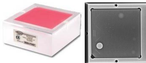
Figure 1. Small ACR mammography phantom and phantom image (Gammex, Inc, Sun Nuclear Company; Model 156)
